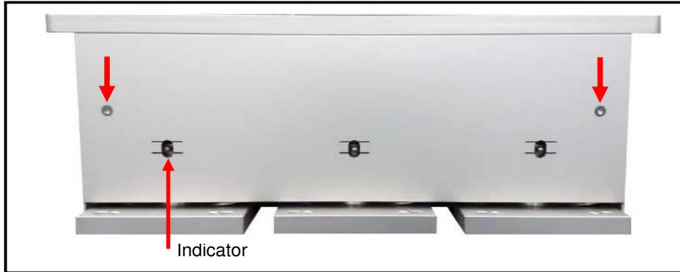
Under load the upper gap and the lower gap shown in Fig. 4 should be approximately equal. (It is however not essential that the gaps be equal - either gap may be as small as 0.5mm without affecting normal operation, but a small subsequent change of load might cause the unit to move against the stop).
