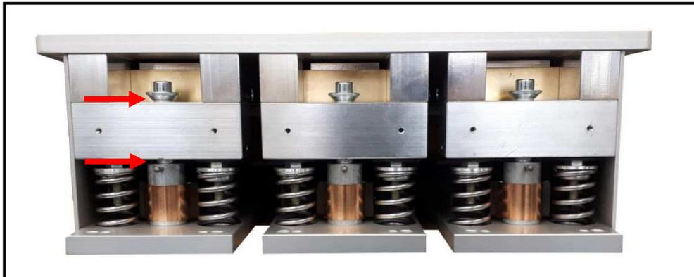
If an adjustment is needed turn the M6 nuts using the spanner provided. Adjust all springs on both sides equally. Moving the spanner to the left raises the units. Use the setting gauge provided to adjust the springs to a gap of max. 13mm. Do not turn the nuts too far or you may damage the units. Under no circumstances should the gap be greater than 13mm.
