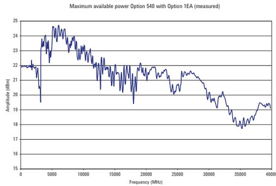
1. Quoted specifications between 15 and 35 °C. Maximum output power typically decreases by 0.2 dB/°C for temperatures outside this range.
