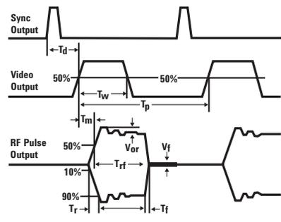
1. Pulse specifications apply to frequencies > 500 MHz. Operable down to 10 MHz.
