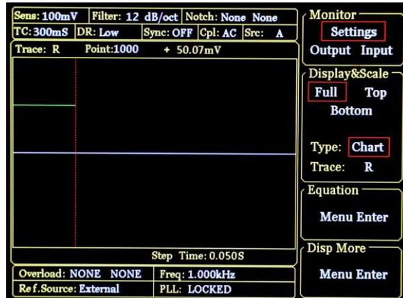
In addition, SE1022 can also use polar coordinates to display the in-phase component and quadrature component of the input signal. All of these display modes can be easily adjusted by manual or automatic operations.
