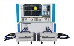
SAV364X Series S parameter test module is a top-level VNA frequency extender. The S parameter test module is used to build a vector network measurement system together with a VNA and a millimeter frequency controller. The system can do millimeter wavelength level S parameter measurement.
