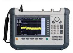
S3301 is an easy-use Handheld Microwave Spectrum Analyzer. With a good performance, S3301 can meet the needs of measurements from short wave to Ku band wave .
