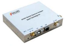
SAV501is a modular spectrum analyzer which can archive the specifications of the main stream spectrum analyzers. SAV501 can be connected to a PC to collect data and display trace/ information. The modular spectrum analyzer also provides USB, LAN interfaces and support SCPI for remote access.
