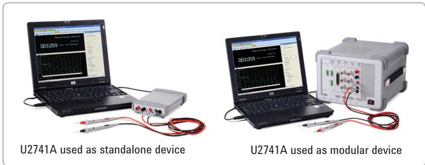
Figure 1. The U2741A DMM showing dual-play capability
