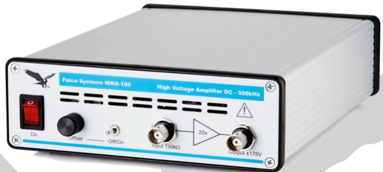
The WMA-100 is a compact all-round, general-purpose high voltage linear amplifier. It offers a wide output voltage range ( $\pm 175\text{V}$ ), DC offset control, and impressive bandwidth (DC - 500kHz) and noise ( $350\mu\text{V}_{\text{rms}}$ ) specifications. The amplifier generates no overshoot with any capacitive load. The short-circuit protection with a fast current limit make this amplifier suitable for both normal daily laboratory use and automated measurement systems.
